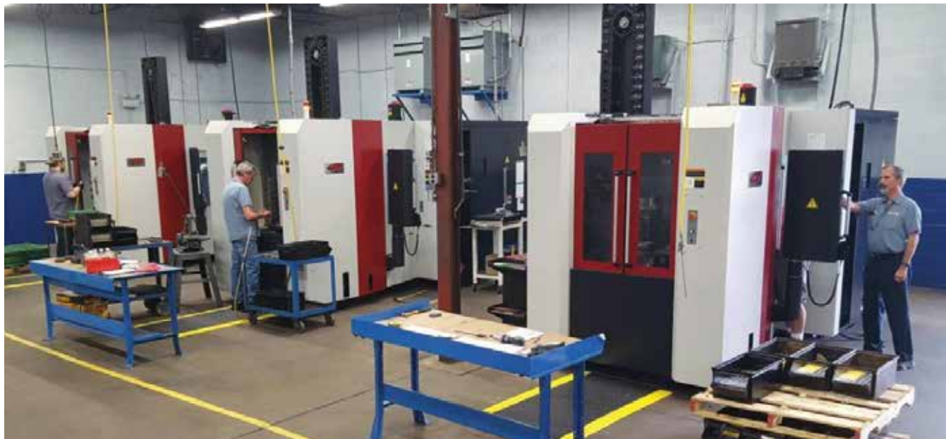
Above: Three SAMSUNG SX 4000 CNC horizontal machining centers at Davlan Engineering in Kirkwood, MO.
